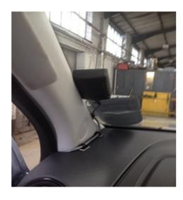
3. The GPS Module should be placed in a suitable area within the cab, preferably in an area next to the windscreen.
