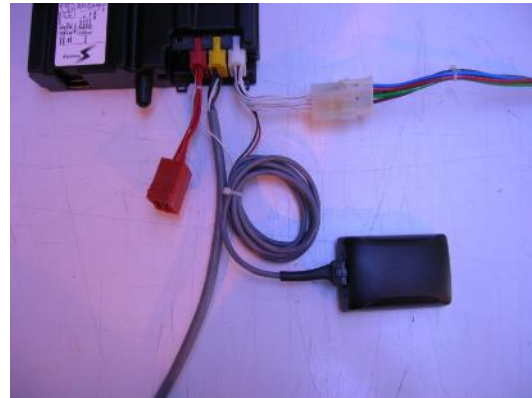
19. The cable harness is connected directly in-line with the tachograph power cable when connecting to the tachograph as shown.
