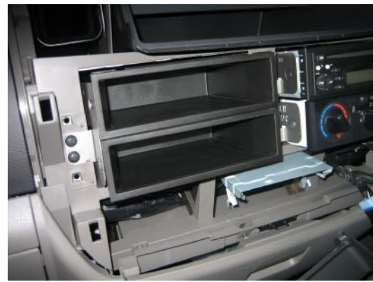
9. Remove the facia around the radio and money tray by unclipping it.
