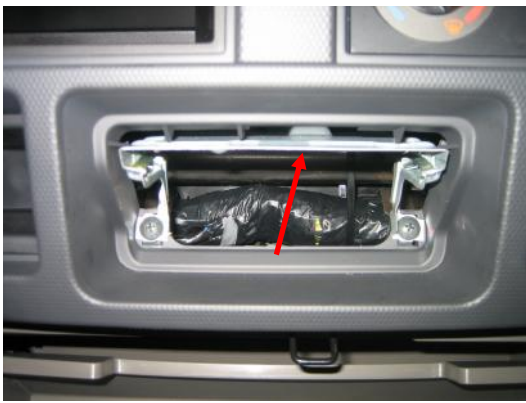
8. Remove the ashtray and the screw which is located on the roof of the securing metal work
