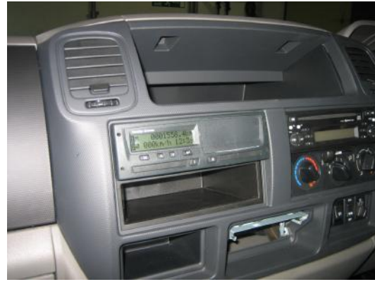
17. The tachograph can now be connected and installed.
