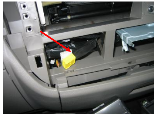
11. Locate cable harness which is secured to the wiring loom behind the ashtray.
