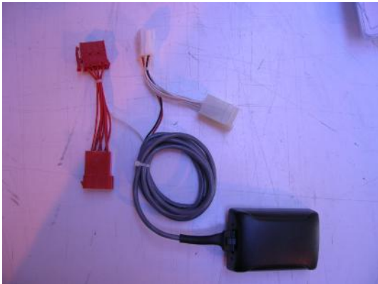
18. The 2nd Source of motion is obtained by using the GPS Module and cable harness as shown.
