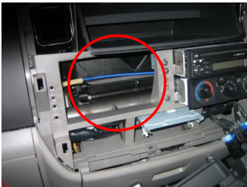
10. Remove the money trays by removing the 2 screws on either side.
