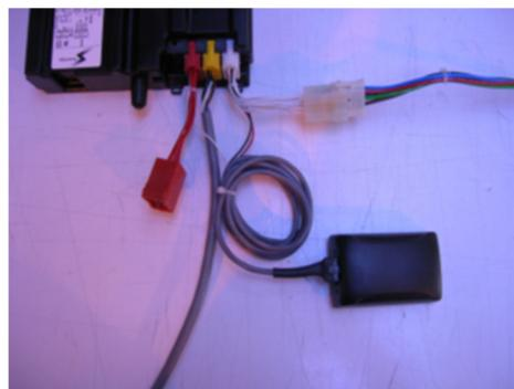
2. The cable harness is connected directly in line with the tachograph power cable when connecting to the tachograph as shown.
