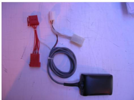
1. The 2nd Source of motion is obtained by using the GPS Module and cable harness, as shown above.
