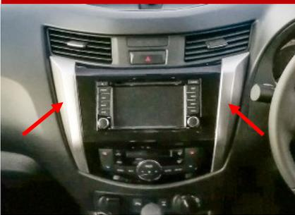
UNCLIP THE SIDE PANELS INDICATED LEFT TO GAIN ACCESS TO REMOVE RADIO. SUITABLE POWER, IGNITION AND GROUND CONNECTIONS CAN BE LOCATED AT THE REAR OF THE RADIO, ENSURE THAT THE POSITIVE FEED TO PIN A1 ON THE SE5000 IS TERMINATED THROUGH 1 AMP FUSE.
