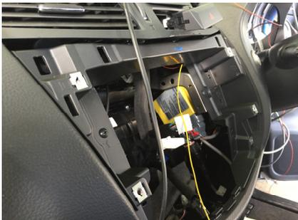
INSTALL THE TACHOGRAPH IN A SUITABLE LOCATION, SEE DVSA GUIDE ON PAGE 3. T-LIGHT MUST BE FITTED AS PER DVSA REQUIREMENTS IF THE VU IS INSTALLED IN A DVSA DESIGNATED AMBER LOCATION.
