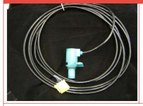
AN ADDITIONAL LINK WIRE IS REQUIRED BETWEEN CONNECTIONS A5 & A6 ON THE VU TO ACHIEVE CORRECT CANBUS OUTPUT.
