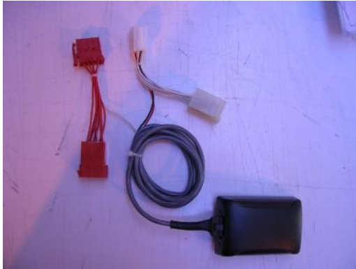
19. The 2 nd source of motion is obtained by using the GPS module and cable harness as shown.
