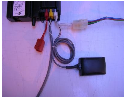
20. The cable harness is connected directly inline with the tachograph power cable.
