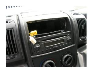
3. Feed the wires from the M1N1 adaptor & the tachograph Power harness through the slot. Mount VU and ensure it can be removed from its enclosure with all cables attached.
