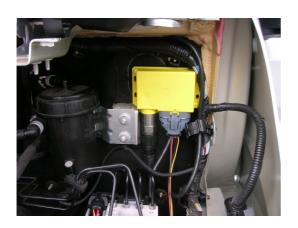
1. Locate and secure the M1N1 adaptor to Near-side rear under bonnet
