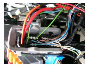
2. Make waterproof connections between ABS Pump Connector Pin 16 Green wire & the M1N1 Yellow wire.
